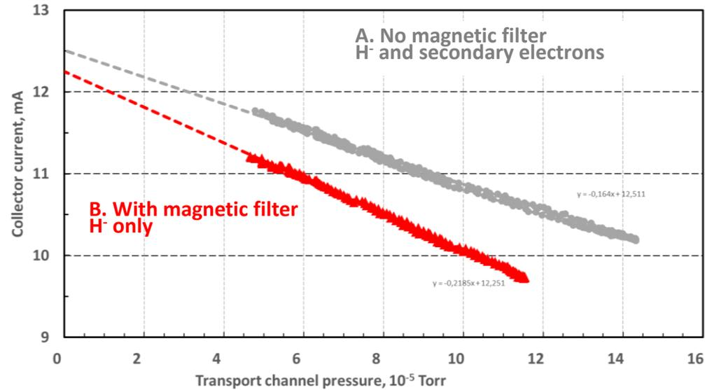
The transmitted current vs the pressure in the transport channel with and without magnetic filter.
