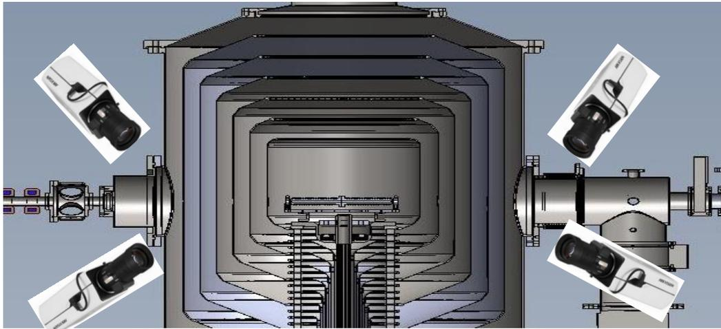
4 CCD cameras observing the entrance and exit apertures are used to record beam position
