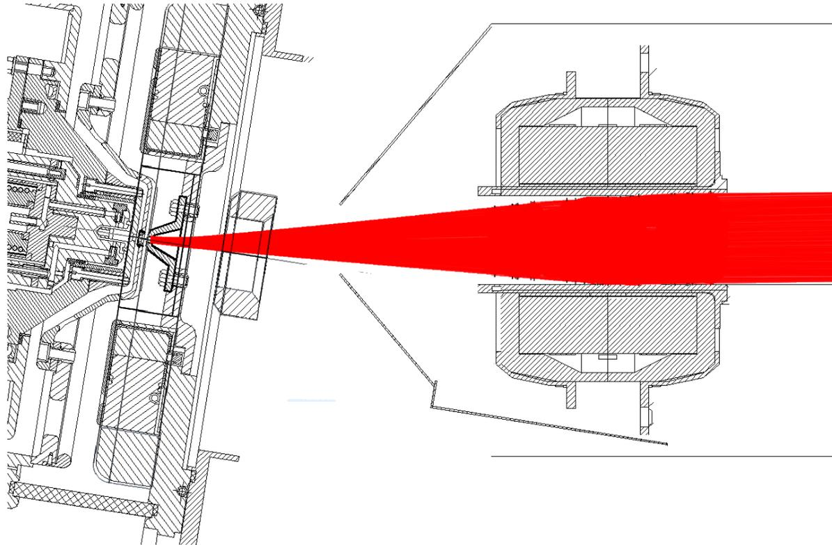
**Calculated negative ion beam trajectories**
