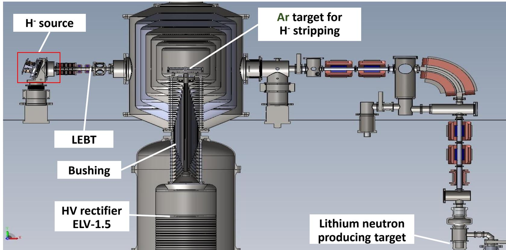
**Tandem VITA is designed for use in the accelerator-based neutron source for BNCT (1998)**
