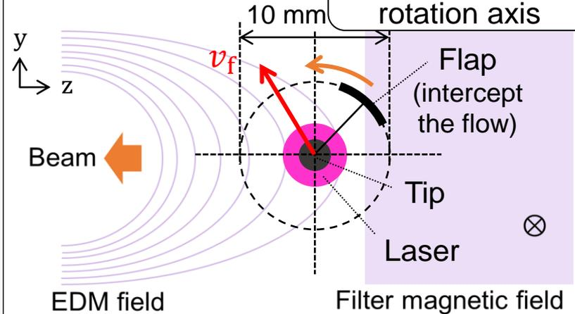
By irradiating laser, this probe works as a directional photo-detachment probe **without the ambiguity to average 4-tip data.**
