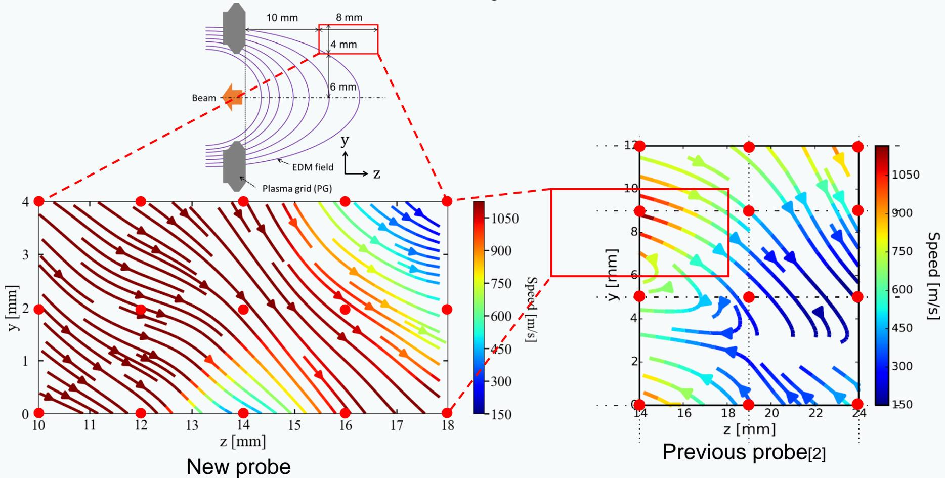
It was verified that the new probe can measure finer flow structure of the charged particles than the conventional one
