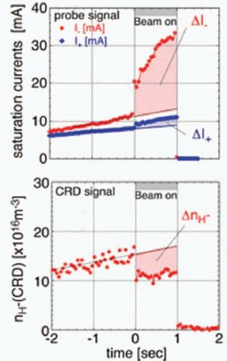
Time evolutions of negative and positive saturation current ( $I_-$ ,  $I_+$ ), and negative hydrogen ion density ( $n_{H^-}$ ) measured by CRD near the plasma grid [1].
