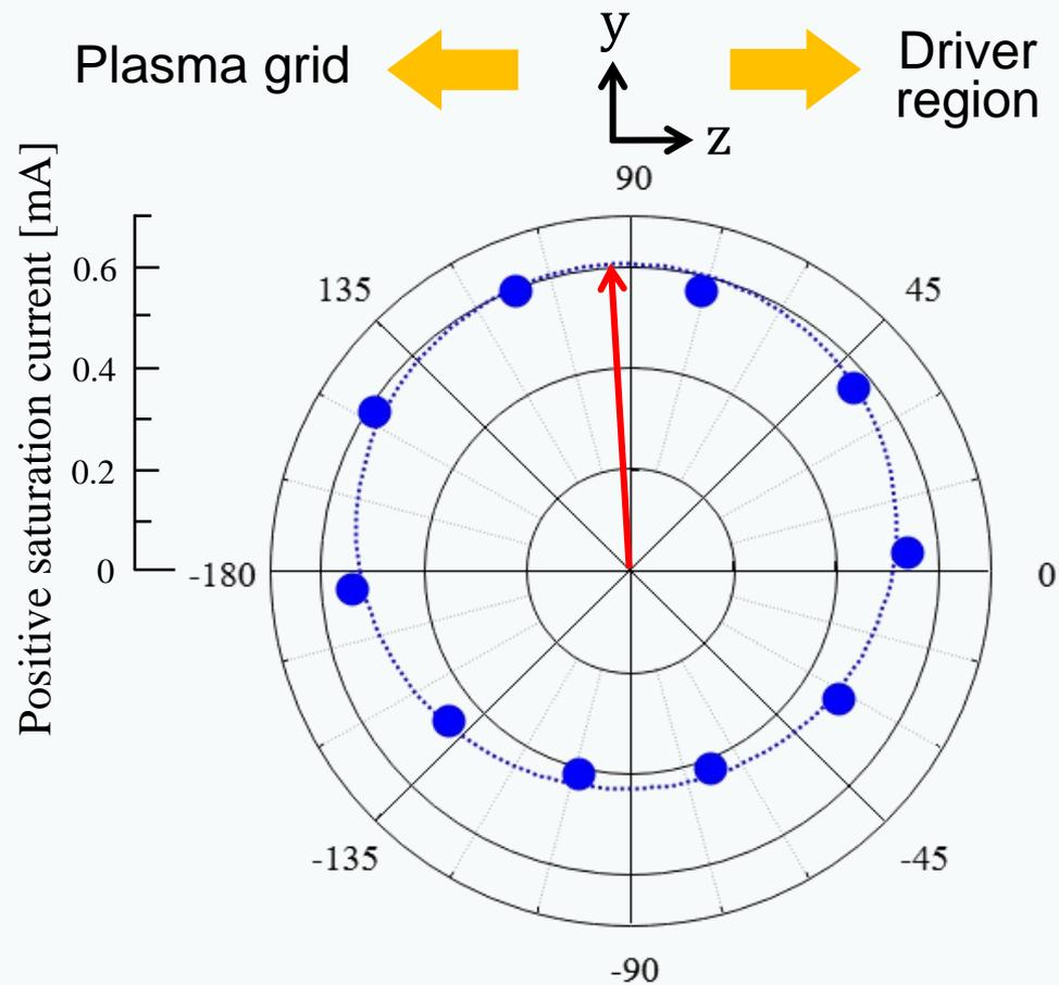
The flow direction is obtained from the positive saturation or photo-detachment currents and the angle of the shielding flap.
