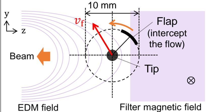
Single probe tip can measure the flow without the density gradient problem.
