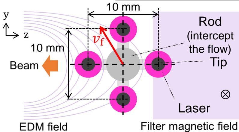
Negative-ion flow is obtained from the signals detected at 4 tips of the Langmuir probe.
