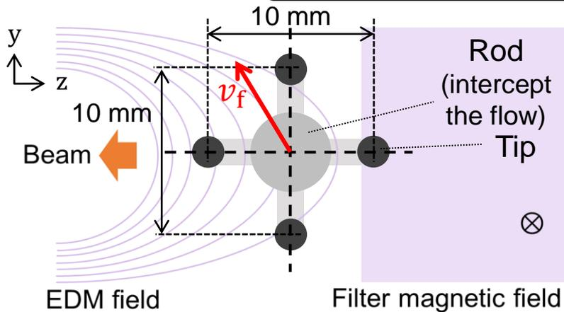
Density gradient between tips can cause error for flow measurement.
