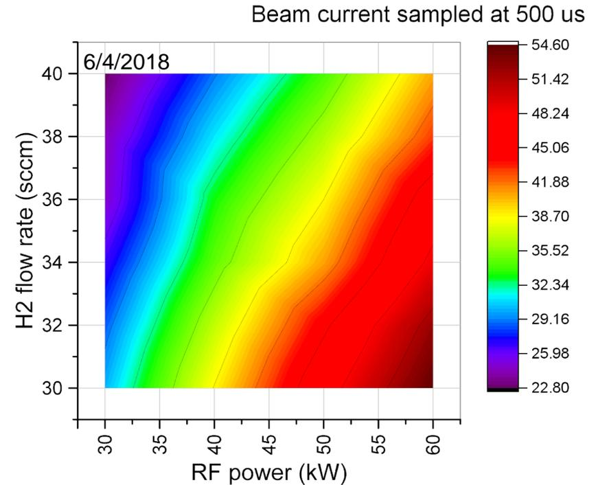
When H<sub>2</sub> flow rate was varied for each power level of 30, 40, 50 and 60 kW, the corresponding beam pulse waveforms were recorded. The plot above is for the beam currents sampled at 500 us from the beginning of the pulses.
