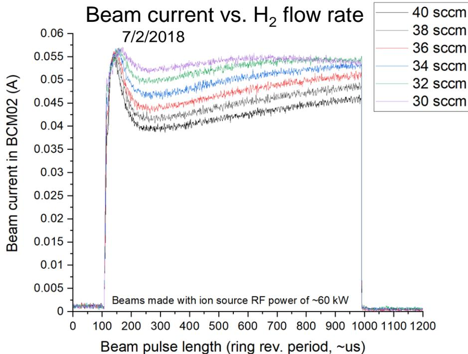
Similarly, the H<sub>2</sub> flow rate was varied for each power level of 30, 40, 50 and 60 kW and the corresponding beam pulses were recorded. The plot above is for the current values sampled at 500 us from the beginning of the pulses.
