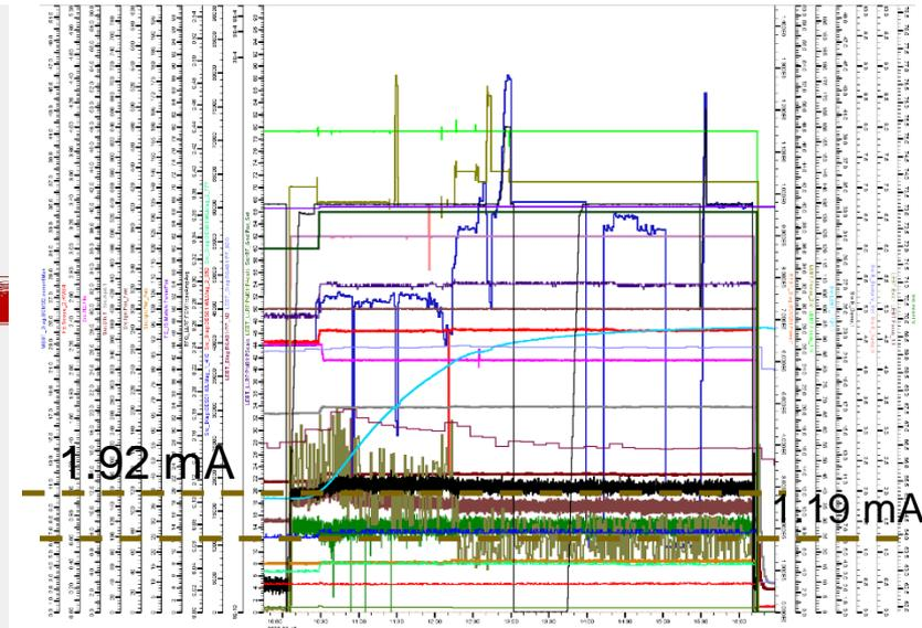
The change of average load current on the extractor electrode:  $1.92 - 1.19 = 0.73$  mA
