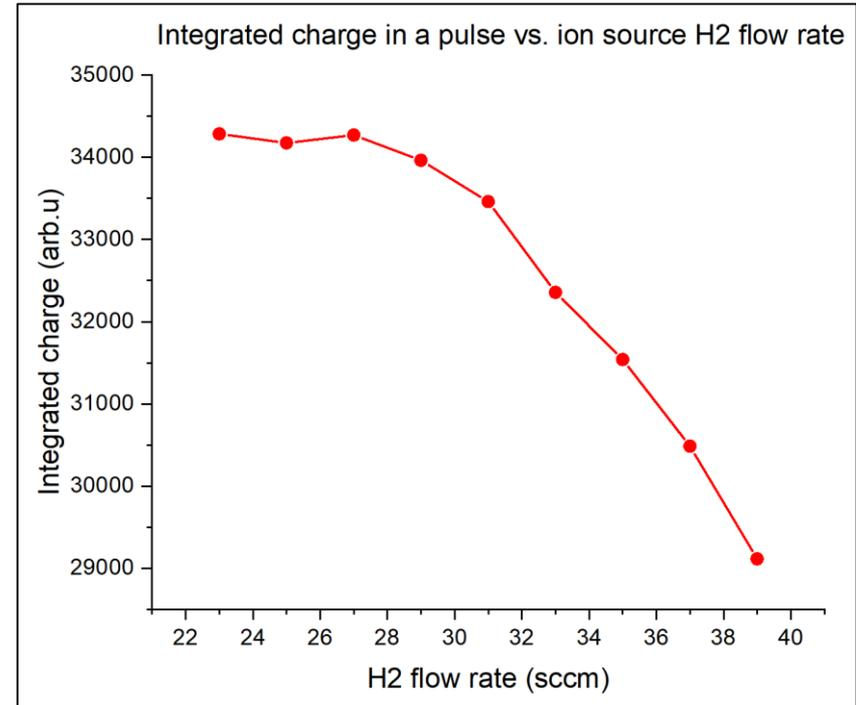
The beam pulse was flatter for the gas flow range of 23-27 sccm, and the integrated charge in a pulse was maximal
