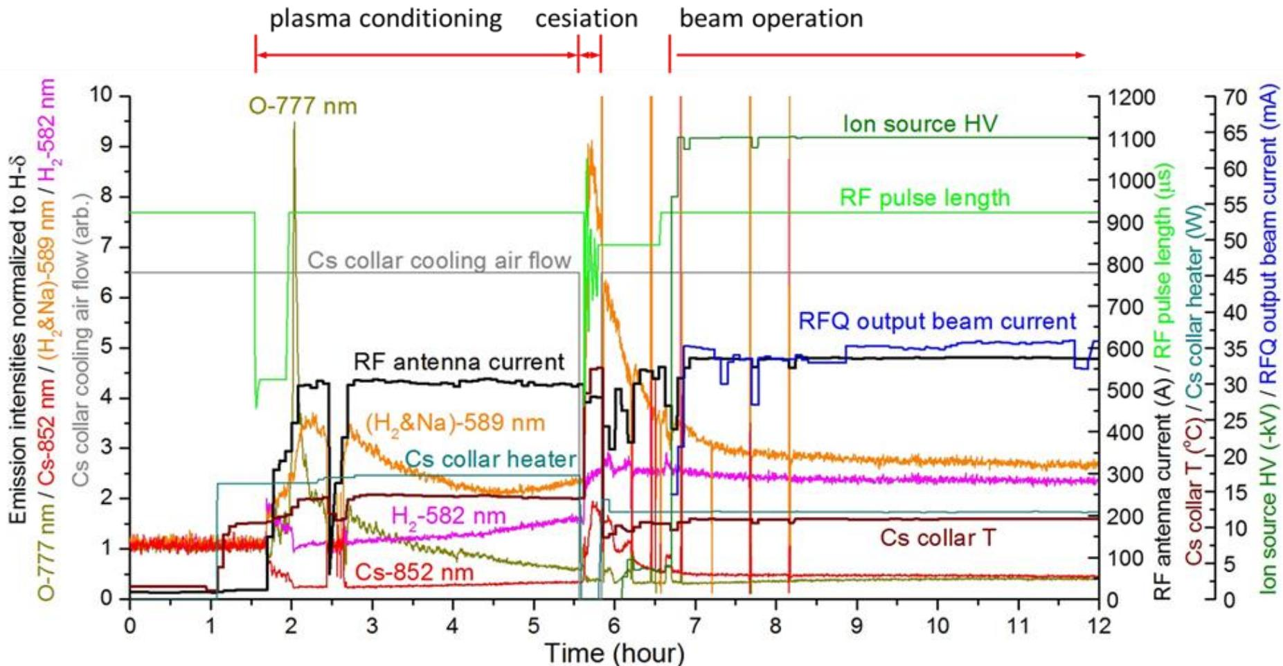
1. The ion source is conditioned with plasma for ~3 hours, which outgases and sputter cleans the system. During the plasma conditioning, the Cs collar temperature is maintained at near 200 °C to help outgassing the Cs collar assembly completely. The Cs collar temperature is controlled by combined effects of RF power, cooling air flow rate and an external heating supplied to the air flow.
