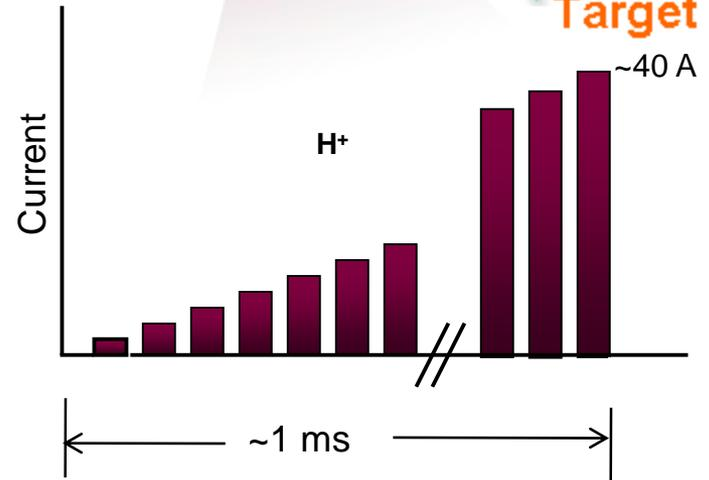
The multi-turn charge exchange injection and low loss beam extraction from the storage ring requires chopped H<sup>-</sup> beam from the linac.
