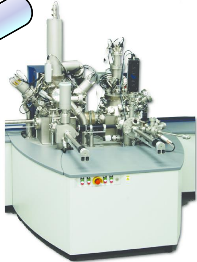
Photo of «TOF.SIMS 5 and Qtac 100» setup, used in LEIS experiments
