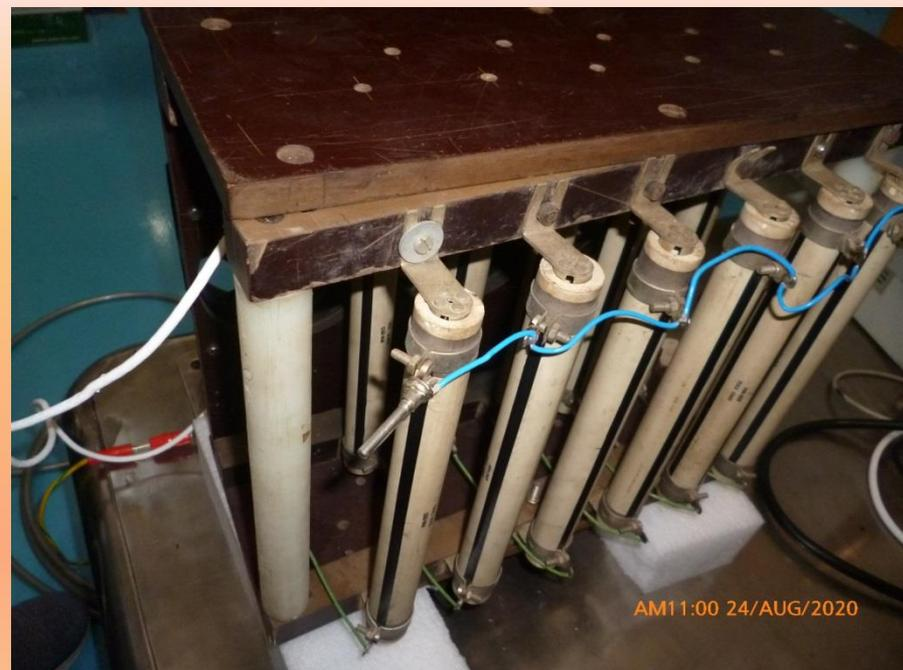
Plasma Electrode (Acceleration) Biasing Network
