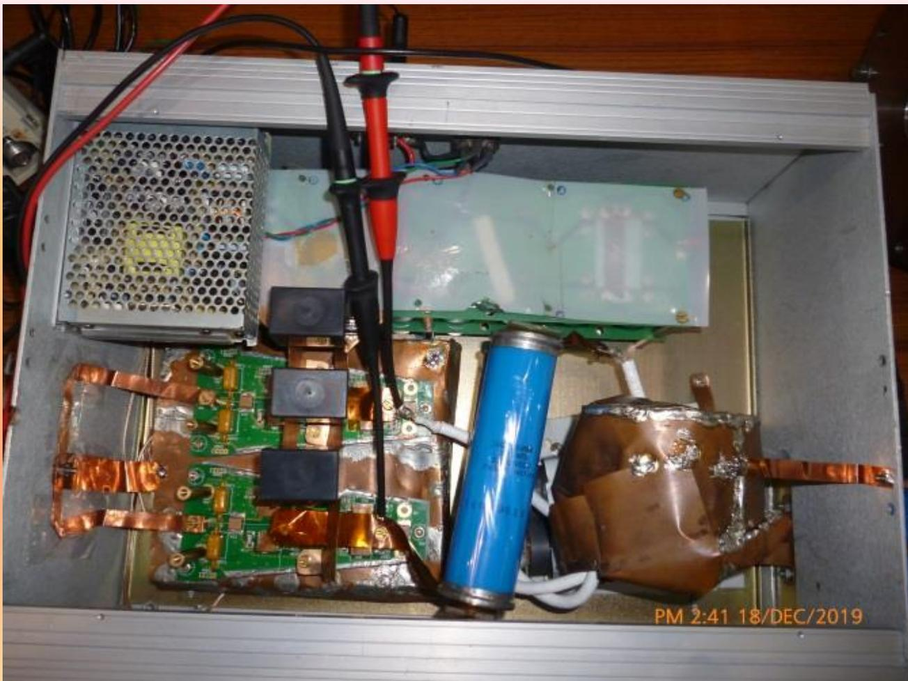
2 MHz Pulsed RF source assembled in 4 U, 19 INCH electronics casing, consisting of DC capacitor bank, SiCMOSFET full-bridge inverter, primary series resonant component and step-down isolation RF transformer.
