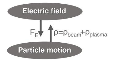
Iteration of electric field calculation and particle tracing.
