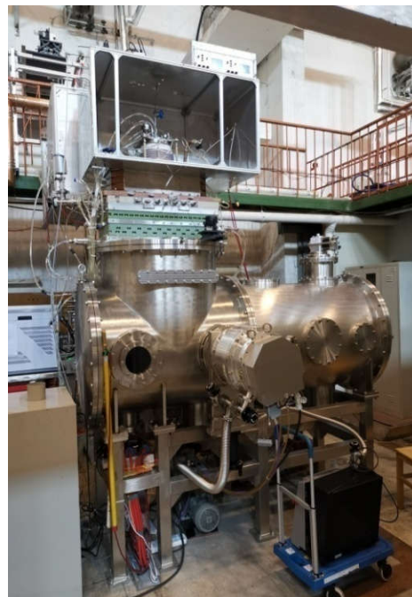
ASIPP NBI test facility of RF ion source
