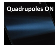
Beam compression is seen by glow in the area between the calorimeter plates taken by bottom CCD
