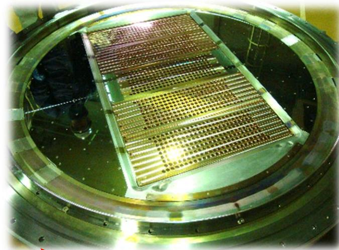
Vacuum insulation design by using meter-class large grid
