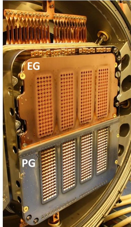
PG and inner surfaces of the ion source are coated with molybdenum to avoid Cs interaction with Cu.
