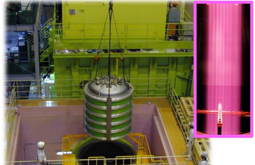
By using 5-stage accelerator, long pulse MeV-class beam acceleration tests over 100 s – 1000 s
