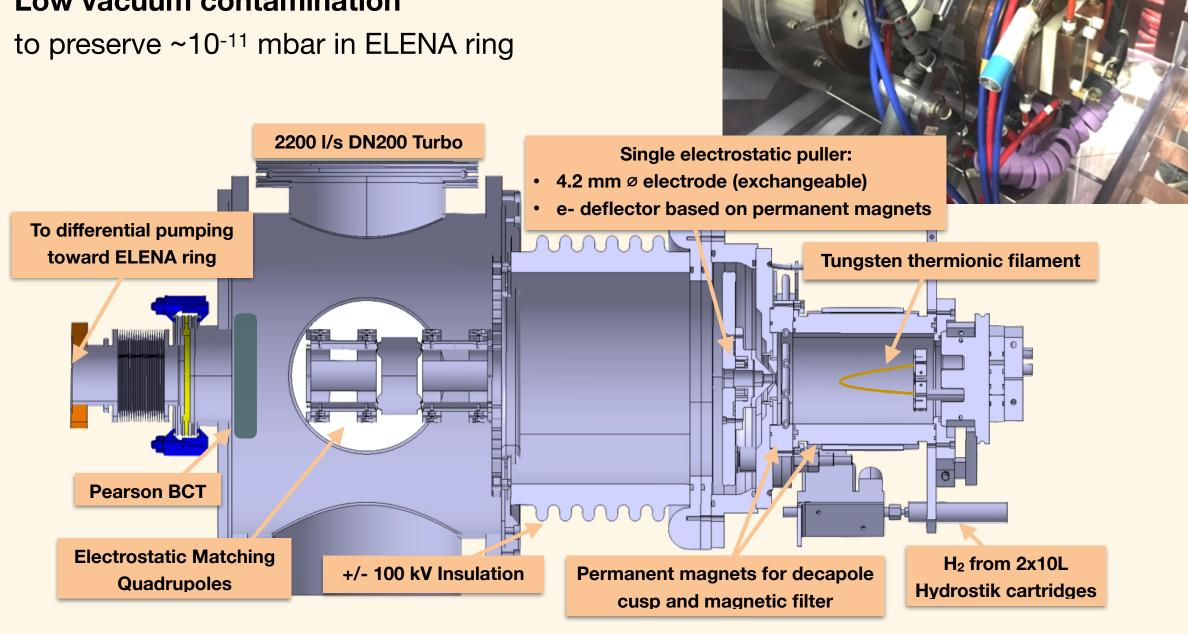
Based on a refurbished and upgraded multi-cusp volume source previously used at the COSY/Jülich injector cyclotron
