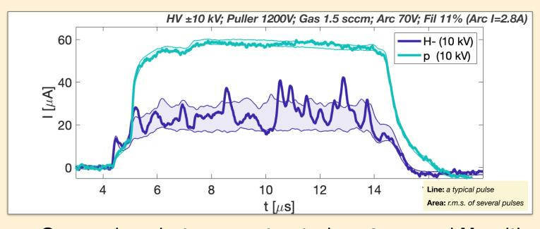
Comparison between extracted protons and H- with the same plasma parameters **points toward** an instability in the H- formation process
