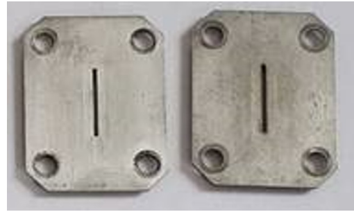
Figure 2. On the left is the standard aperture plate, 0.6 mm x 10 mm, to compare with the double width aperture plate on the right, 1.2 mm X 10 mm. The double width aperture plate was used to increase the beam extracted in long pulses.
