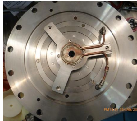
FIGURE 3. (a) The 2D-CAD drawings of extraction electrode, and (b) The photograph of extraction electrode with water cooling arrangement.
