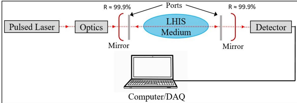
**FIGURE 2.** Basic setup of the diagnostics. Removing (Adding) the Mirrors gives LAT (CRDS) setup.
