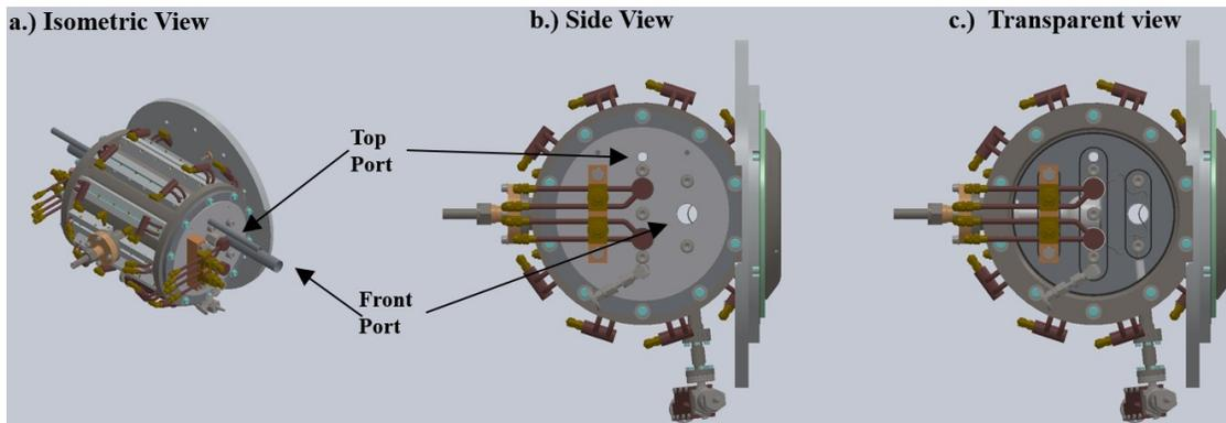
**FIGURE 3.** The first modification LHS with side-plate ports installed. The right view (c) gives a transparent view, where side plate is transparent so that underlying vacuum and water cooling O-rings are shown. Cesium density will be measured using both the top and front ports. The  $H^-$  density measurements will be measured using the front port, with the ability to take several data points within the port.
