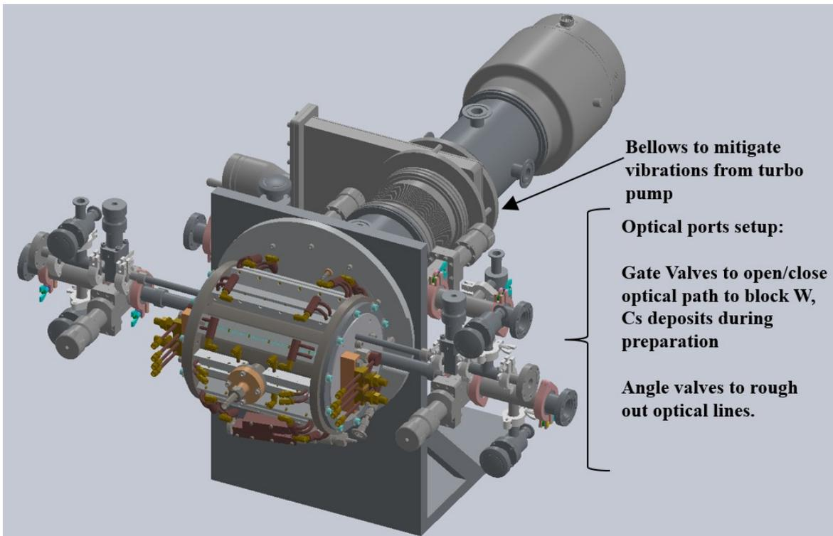
**FIGURE 4.** The laboratory setup. The main challenges addressed by this setup are given in the text in the figure.
