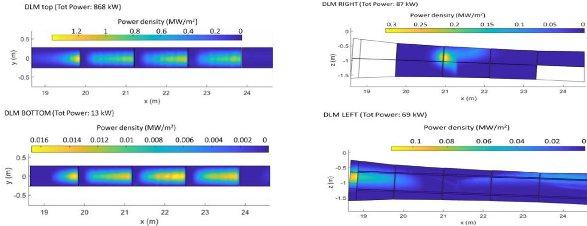
**FIGURE 8.** 2D views of the power loads at DLM panels for the scenario D 7, -2, +10, FFFC
