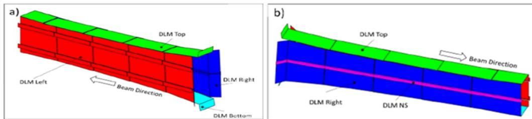
**FIGURE 4.** MATLAB generated view of the surfaces of the DLM: **54 surfaces**, including two surfaces mimicking the DLM opening towards the neutron shield (DLM-NS) area behind the duct liner
