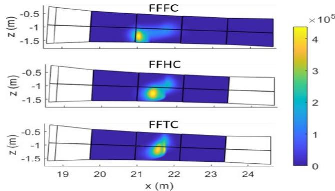
**FIGURE 6.** Power loads on the Right surfaces of the DLM - for three options of the magnetic field. *Deuterium*.
