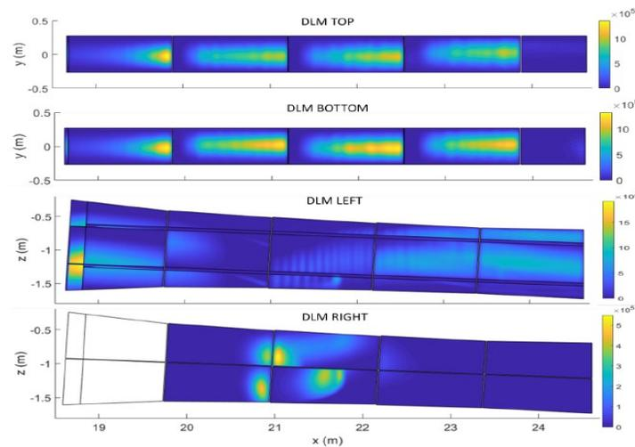
**FIGURE 9.** 2D views (XZ and XY planes) of the maximum power loads at each DLM panel throughout all the scenarios
