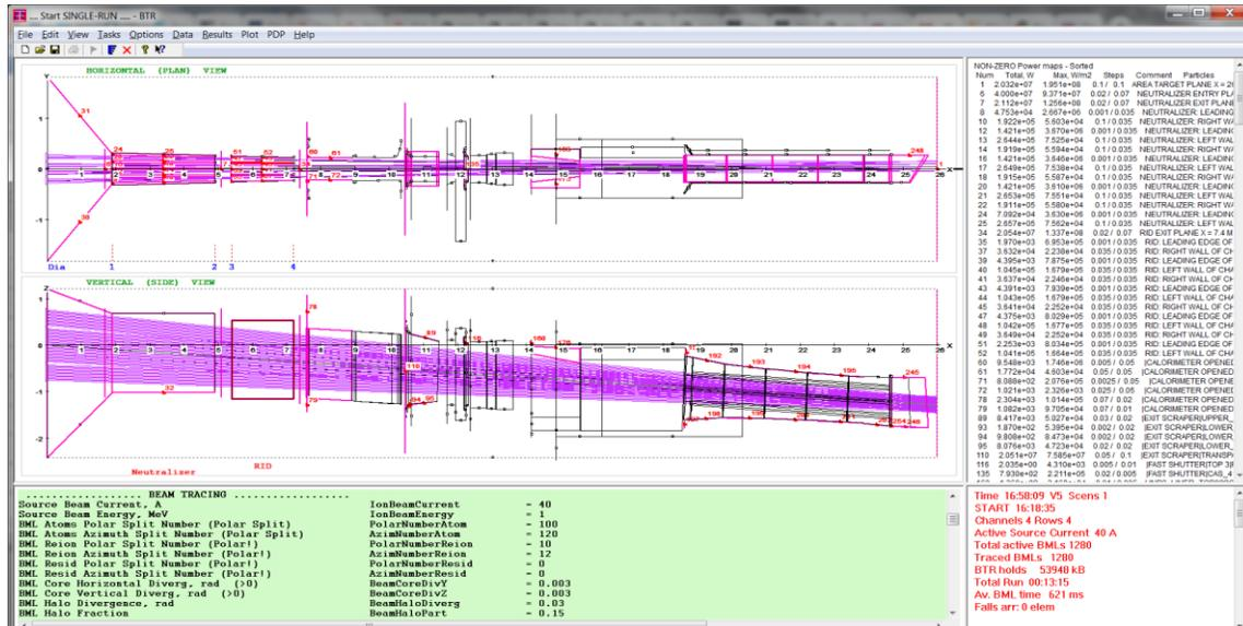
**FIGURE 2.** BTR Screen with ITER HNB geometry: horizontal and vertical plane views. Standard NBI geometry is combined with Free surfaces import, which begins from the Calorimeter ( $x = 7.6\text{m}$ ). Beam model is Standard, i.e. defined by regular array in Config-file. The beamlets axes are shown violet. Result power maps Summary (text) is shown top-right.
