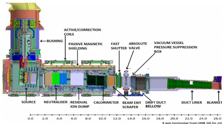
**FIGURE 1.** Sectional view of HNB beam line, taken from [3]
