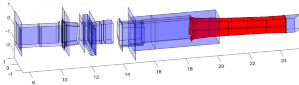
**FIGURE 3.** MATLAB generated view of the CAD surfaces imported by BTR as TXT-files. From the left to right: Calorimeter, Exit Scraper, Fast Shutter, Absolute Valve, Drift duct liner, connecting duct, and the duct liner DLM (red).
