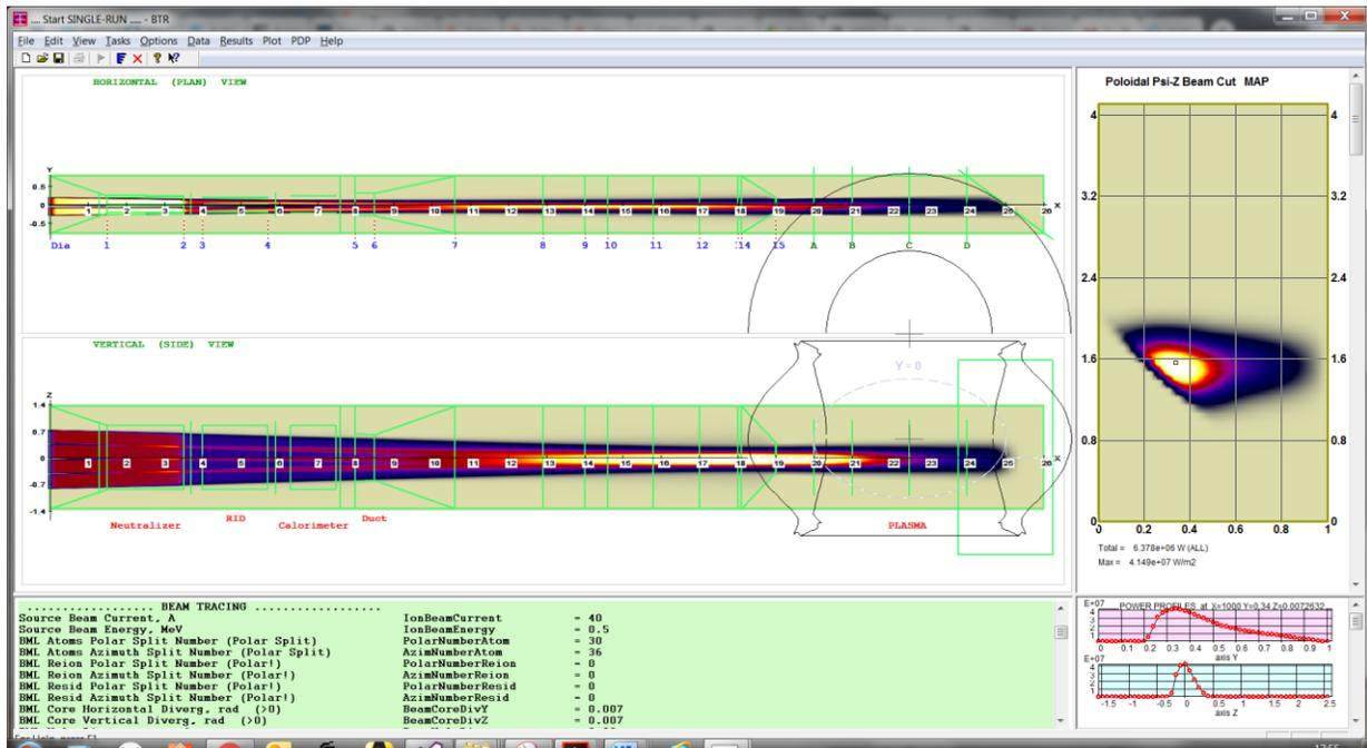
FIGURE 2. BTR-code Screen with the beam power cuts in horizontal and vertical planes (DEMO-FNS NBI)
