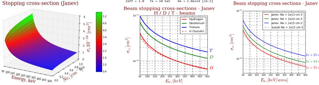
FIGURE 3. Effective stopping cross-section calculated by BTOR (Python). DEMO-FNS:  $\sigma_s = 0.9 - 1.2 \times 10^{-20} m^2$
