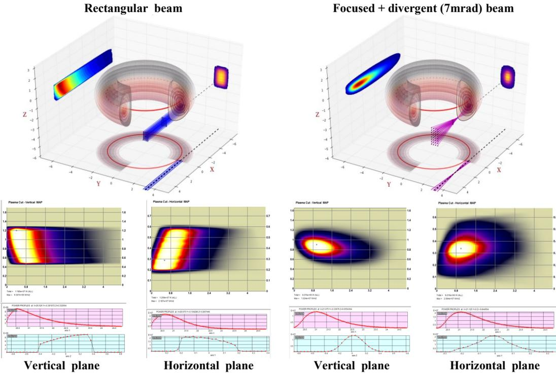
FIGURE 4. Comparison of beam 3D deposition (ionization) for basic neutral beam shapes
