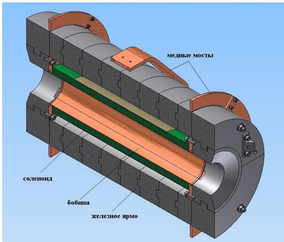
Liquid-free superconducting 6 T solenoid
