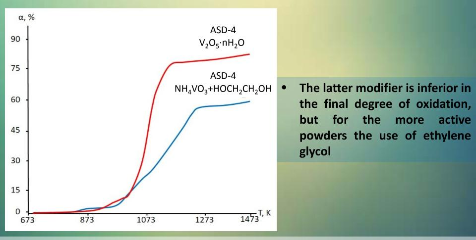
The reduction of the degree of conversion can be due to the decomposition of a more complex modifier based on ethylene glycol and ammonium metavanadate because in this case expenditure of energy is required. Active pentoxide appears on the diffraction patterns only above 673 K.
