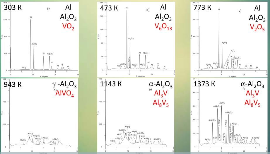
The variety of processes taking place almost simultaneously in the volume and on the surface of the sample, which is due to vanadium polyvalence, as well as the low temperature destruction of the oxide shell promote efficient transport of oxidant (oxygen) to the metal surface.
