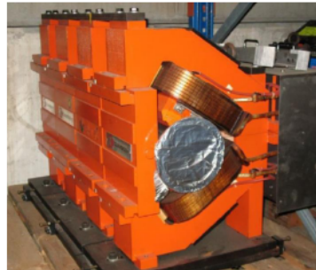
Robinson wiggler in PS Ref: Emittance control of the PS e + beams using a robinson wiggler, Y. Baconnier et al.
