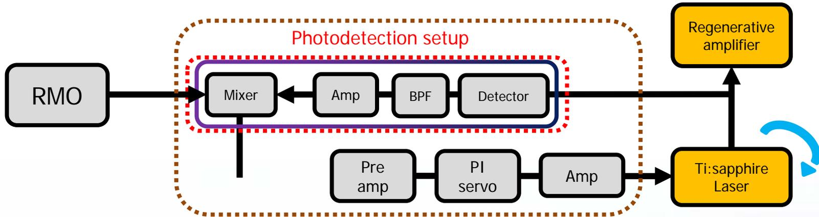
FLOM-PD (Frequency Loof Optical Modulation – Phase Detector)
