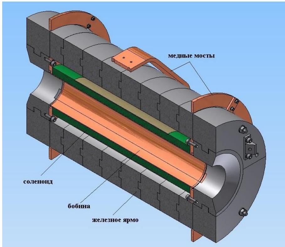
Liquid-free superconducting 6 T solenoid
