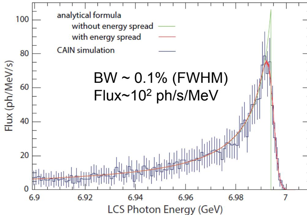
Energy is tunable by changing e-beam energy with keeping X-ray oscillation.
