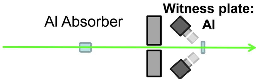
Al witness target chosen as it has strong resonance at similar energies to  $^{239}\text{Pu}$
