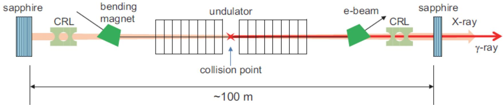
X-ray oscillator with Bragg mirrors (perfect crystals)
