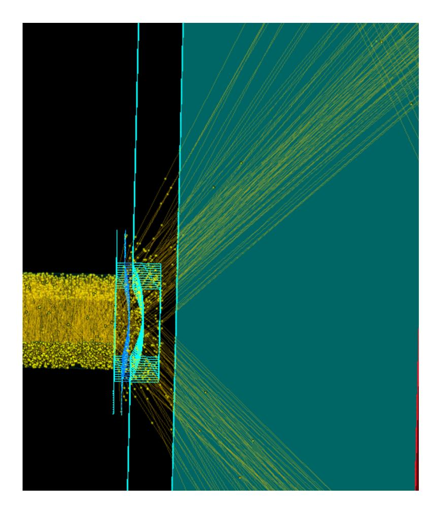
Here zoomed area shows the 3 Layer focusing Lens with circa 20mm thickness all together, again with MC photons
