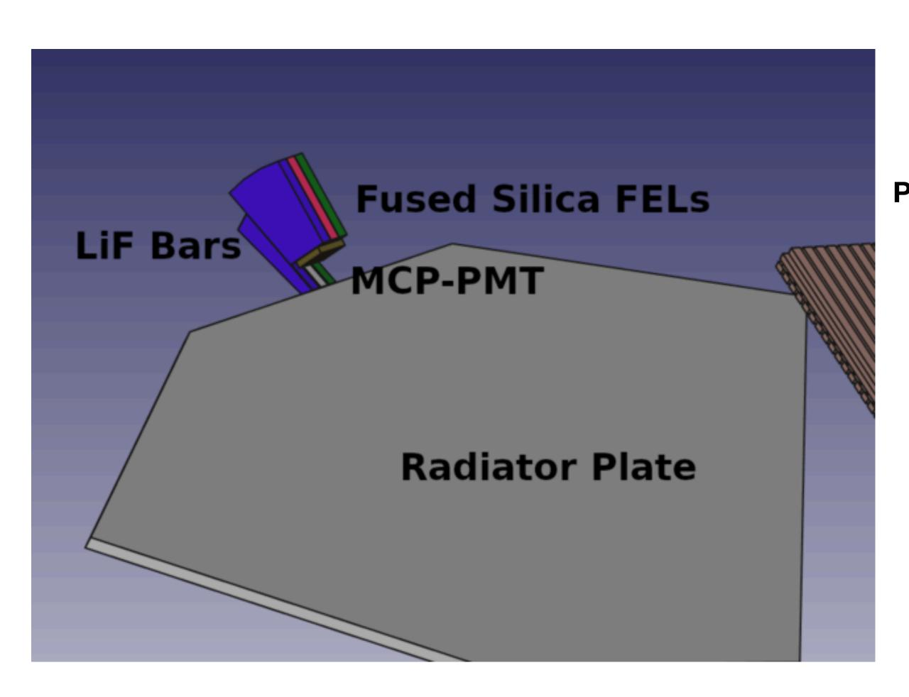
This prototype is now inside GCS and taking data using cosmic muons, the difference from SCTF desired prototype is that, instead of LiF bars, it equipped with SiO2 bars like the Plate and the Photon detector is 300 channel MCP-PMT instead of SiPM
