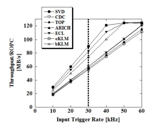
➤ Throughput is saturated due to the limit of output GbE bandwidth.
