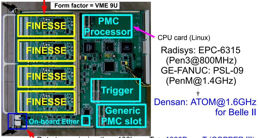
Data transmission thru. 100base-T -> 1000Base-T (COPPER III)
