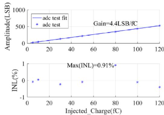
$$\text{Gain} = 4.4 \text{ LSB/fC} = 4.4 \times 2.34 \text{ mV/fC} = 10.3 \text{ mV/fC}$$
