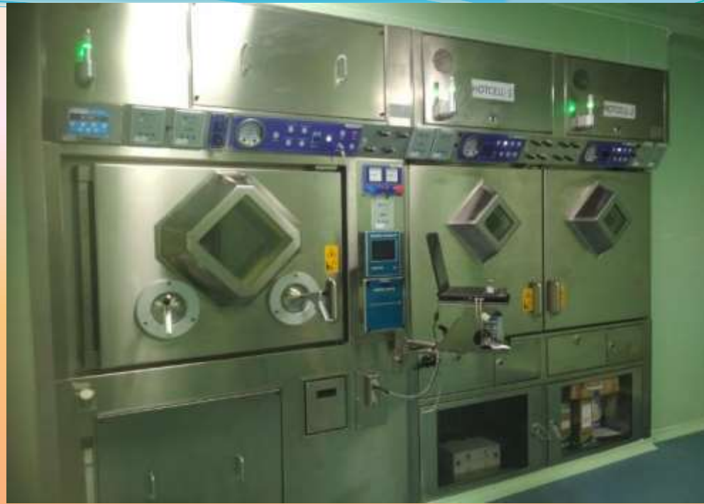
PET Hot cells for production & dispensing of ^{18}\text{F} -FDG
