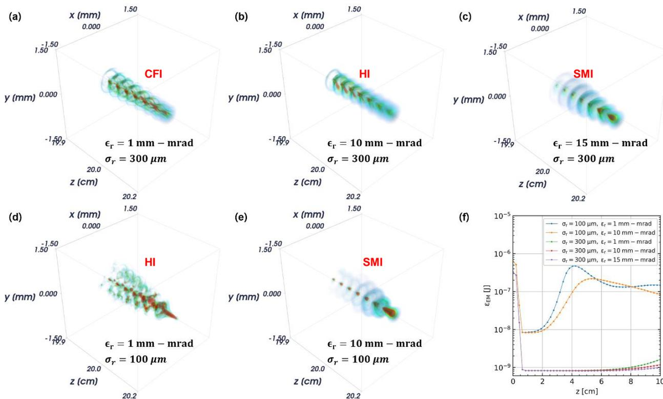
Beam-plasma instability can be selectively induced by adjusting beam radial size and transverse emittance.
