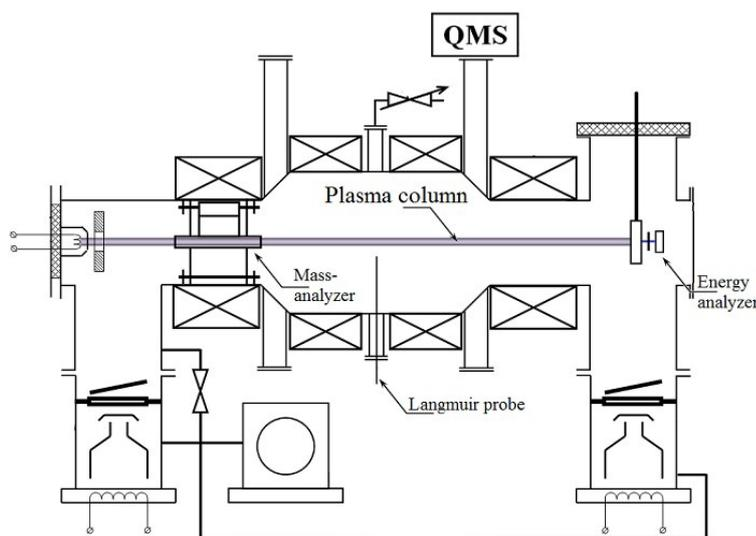
Figure 1: Scheme of linear plasma device PR-2
