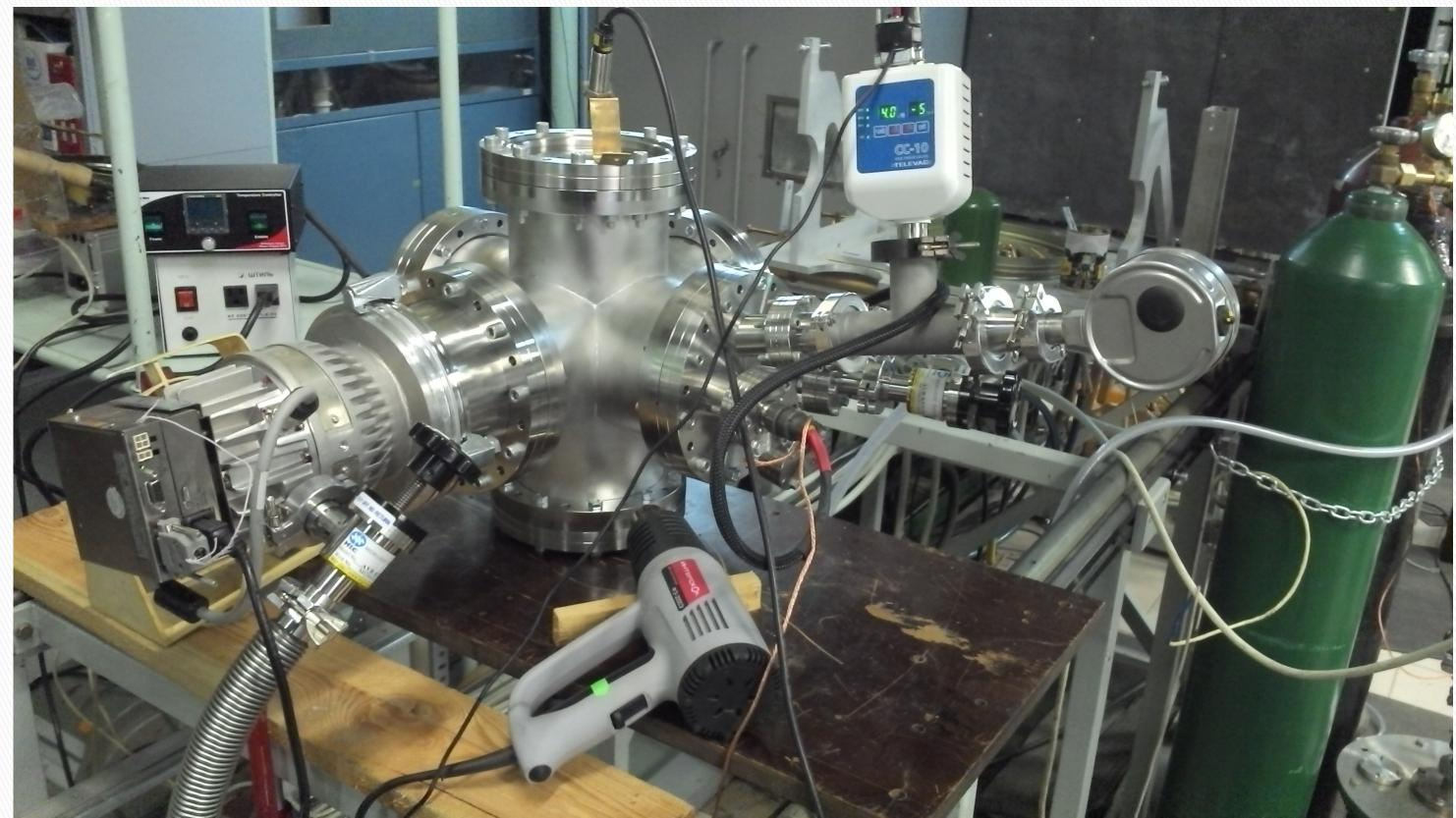
• High vacuum down to 10<sup>-6</sup> Torr • Hydrogen/deuterium pressure up to 2 bar
