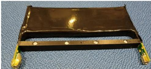
Two scintillator tiles (12 cm x 4 cm), placed upstream and downstream of the drift tubes pack, instrumented with SiPM.
