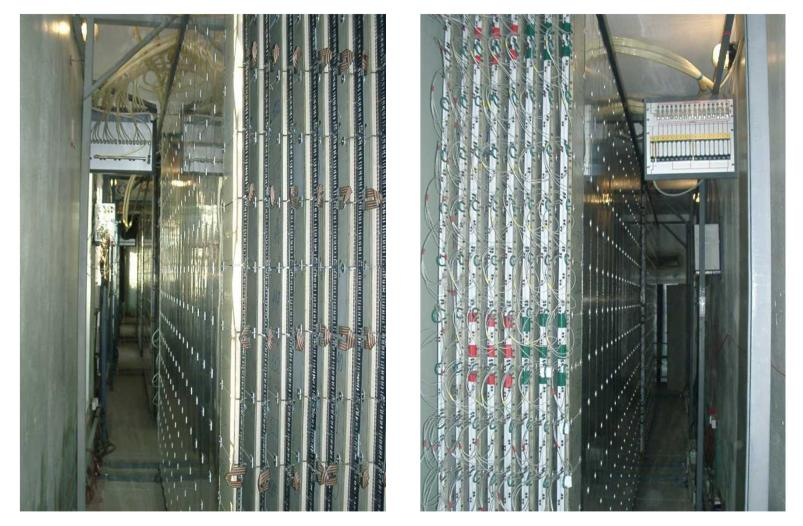
Each SM has an effective area 8.4 m<sup>2</sup> and consists of 8 planes of streamer tube chambers. The length of the chambers is 3.5 m, inner tube cross section is 9×9 mm<sup>2</sup>. The planes of the chambers are equipped with a two-dimensional system of external readout strips.
