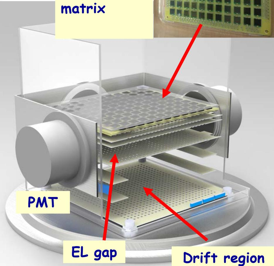
The cryogenic chamber included a cathode electrode, two field-shaping electrodes, a THGEM0, immersed in liquid Ar layer and a double-THGEM assembly, consisting of a THGEM1 and THGEM2, placed in the gas phase above the liquid.
