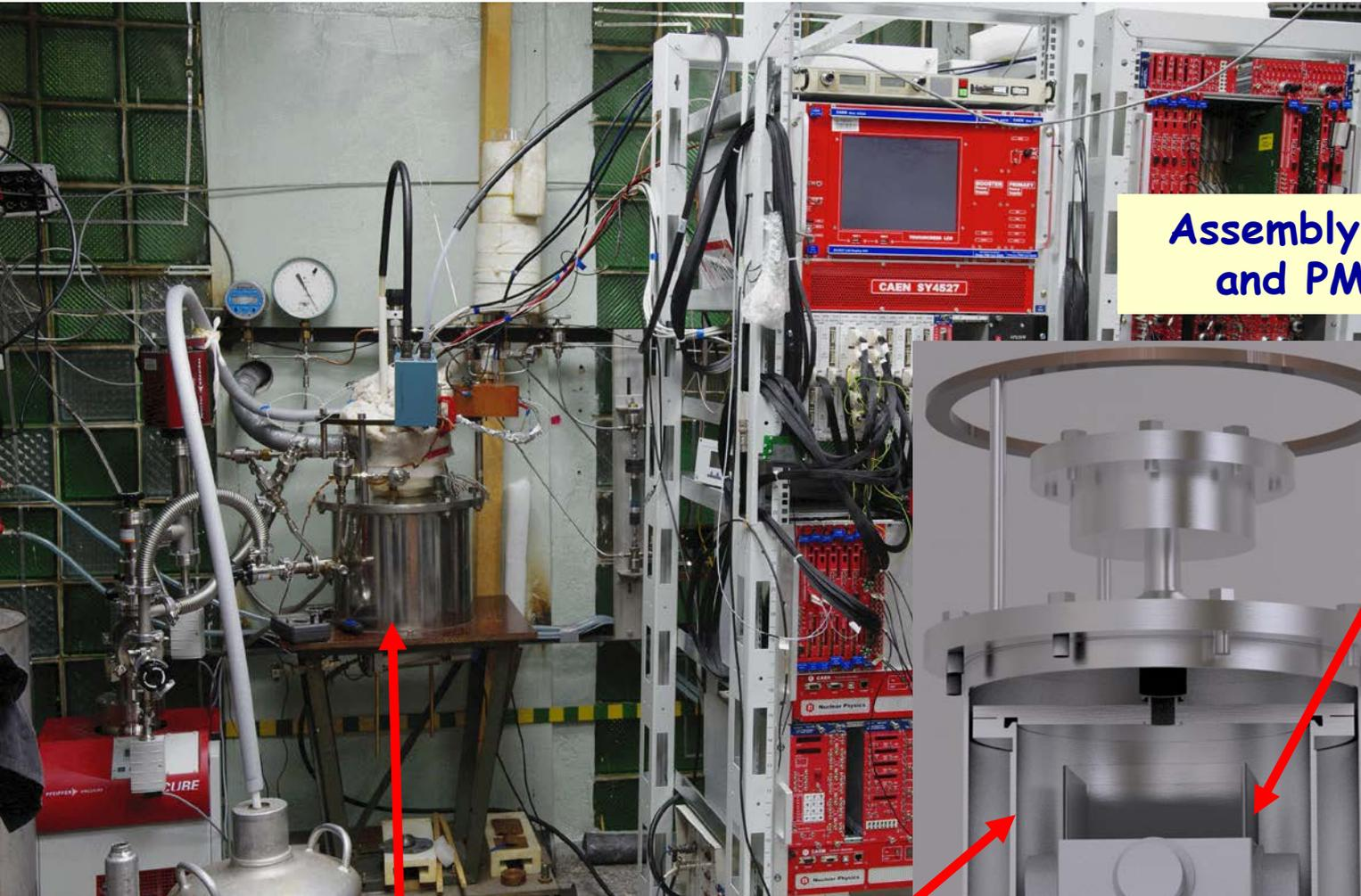
Assembly with EL gap and PMT readout
