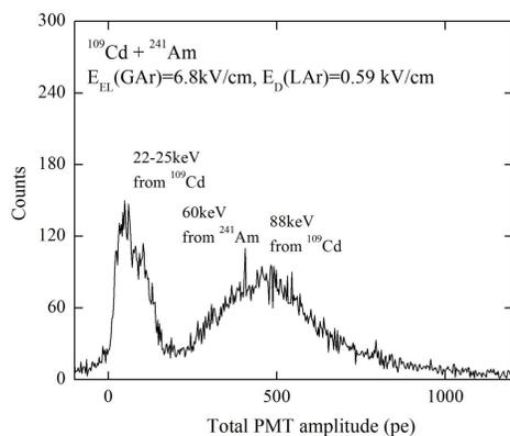
Amplitude distribution of the total PMT signal from the EL gap at an electric field of 6.8 kV/cm in the EL gap and 0.59 kV/cm in the drift region, under irradiation with X-rays from  $^{109}\text{Cd}+^{241}\text{Am}$  radioactive source.
