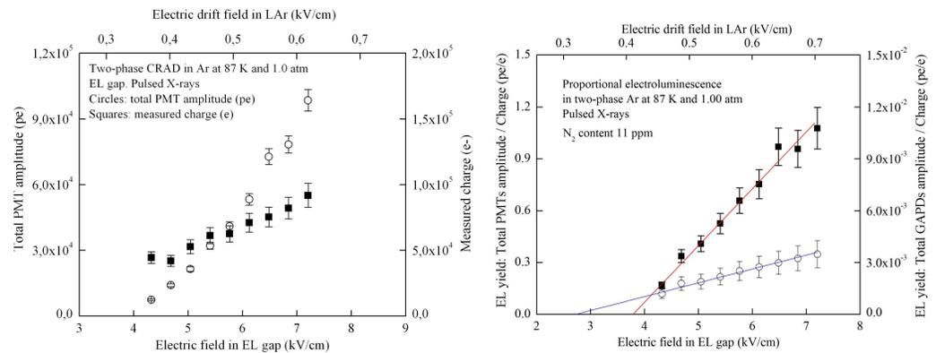
Left figure shows the PMT amplitude in number of pe (circles) and charge in number of electrons (squares) as a function of the electric field in the EL gap. Right figure shows EL gap yield measured using PMT (squares) and SiPM (circles) signals as a function of the electric field in the EL gap.
