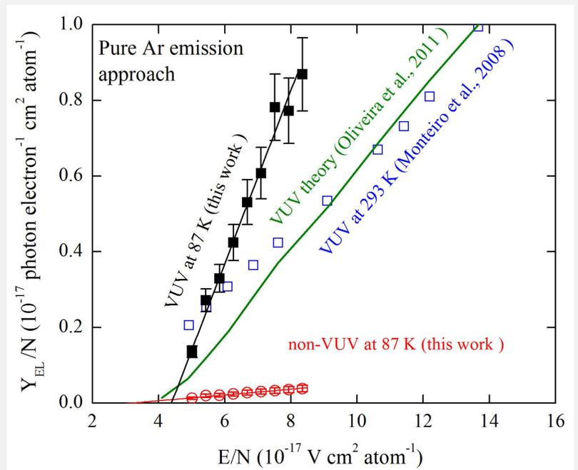
Reduced electroluminescence yield as a function of the reduced electric field in the VUV (Ar emission) and in non-VUV (modeled as  $N_2$  2PS emission), determined in this work in gaseous Ar, in the two-phase mode at a temperature of 87 K and pressure of 1.00 atm. For comparison, the yields in gaseous Ar in the VUV obtained experimentally at 273 K (Monteiro et al.) and theoretically (Oliveira et al.) are presented.
