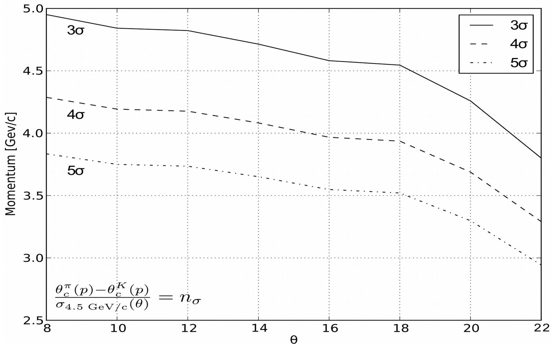
4  $\sigma$   $\pi$ -K separation power @ 4GeV/c up to 18 degree.
