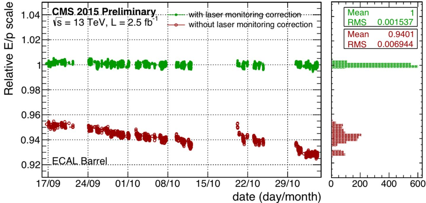
The ratio of electron energy  $E$ , measured in the ECAL Barrel, to the electron momentum  $p$ , measured in the tracker:
