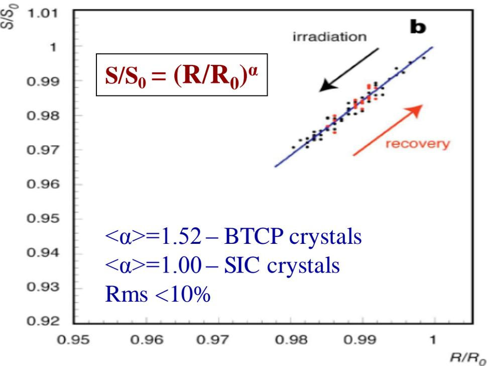
The changes in the crystal transparency due to irradiation impact on the signals from an electromagnetic shower in different way than from laser pulse.
