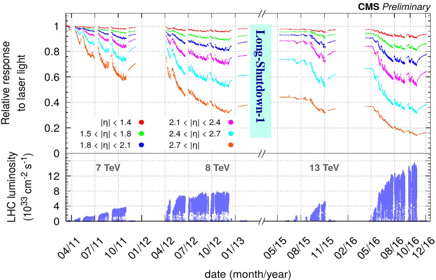
Relative response to laser light averaged over all crystals in bins of pseudorapidity ( $\eta$ ), for the 2011, 2012, 2015 and 2016 data taking periods, with magnetic field at 3.8 T:
