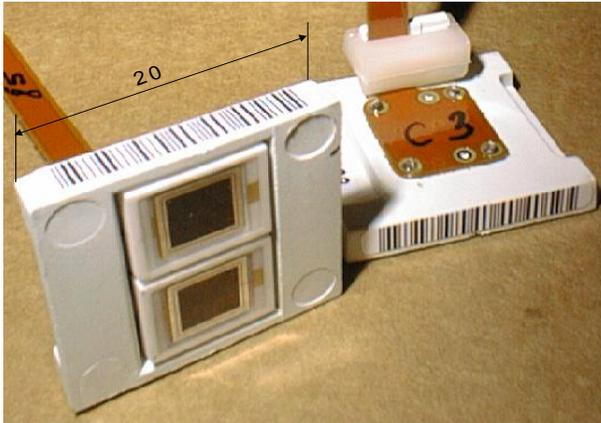
**Barrel:** Avalanche photo-diodes (APD, Hamamatsu)
