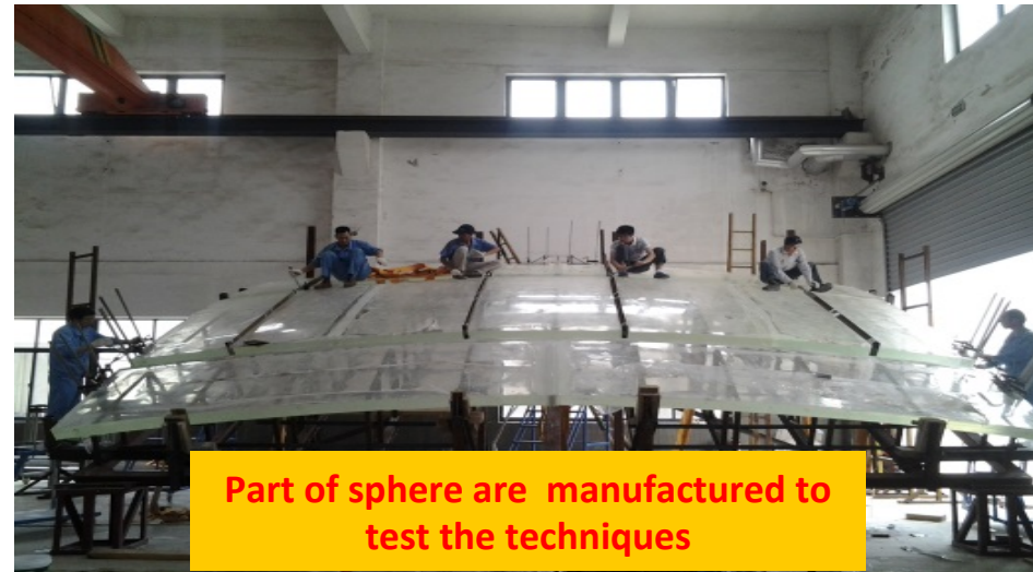
Sphere sheet manufacturing: 3m X 8m X 0.12 m The problems of shrinkage and shape variation were resolved.
