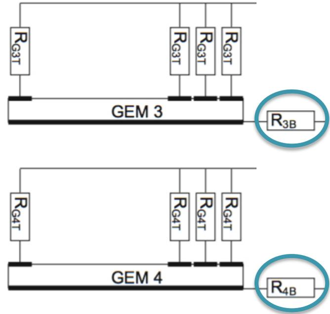
➤ **The onset field for secondary discharges increases with increasing decoupling resistance**
