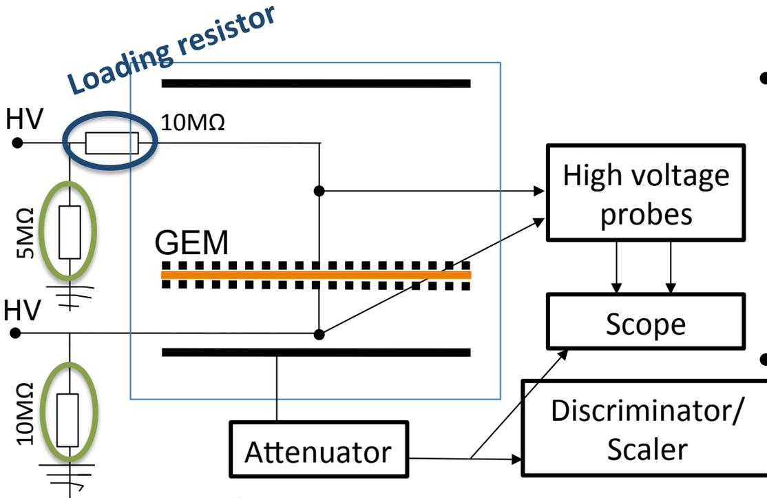
Resistors to sink currents during a discharge
