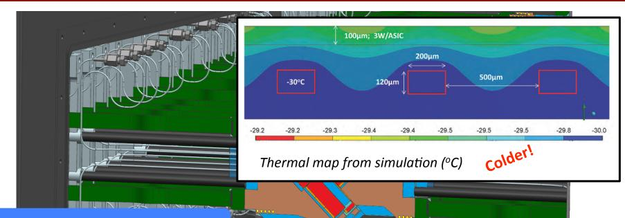
Sensors and read-out electronics mounted on cooling substrate etched with CO<sub>2</sub> micro-channels
