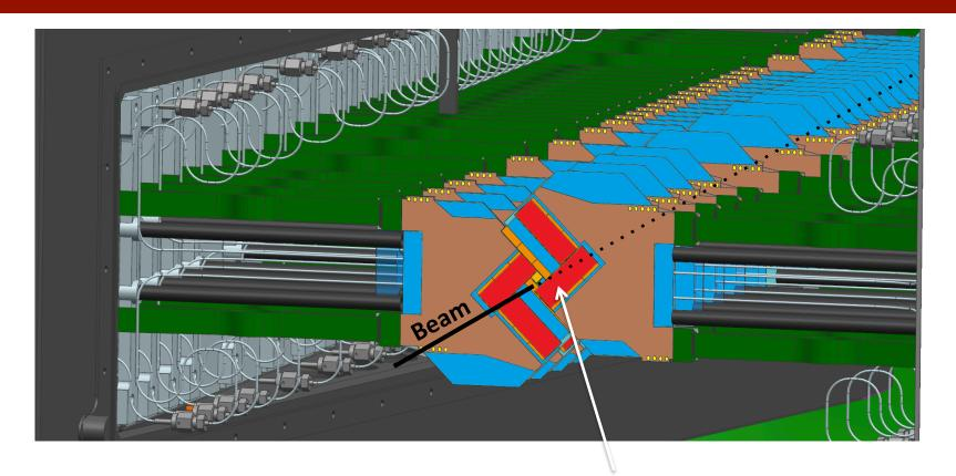
52 modules in total (26 per half), perpendicular to beam
