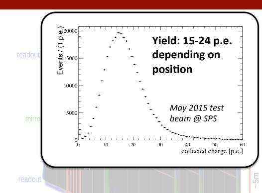
Light collected by 50μm pitch SiPMs, cooled to -40°C to reduce dark counting rate.
