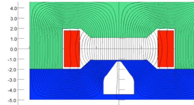
TD:FNAL FEM 2D simulation of the G-2 experiment Lambertson Magnet
