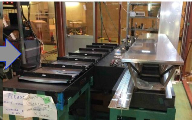
Optics: alignment, gluing, curing and aging (~2 weeks).
