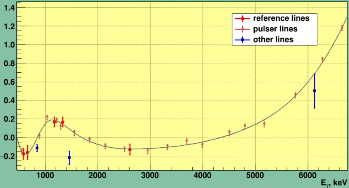
Use of pulser eliminates the MCA nonlinearity down to  $\lesssim 50$  ppm
