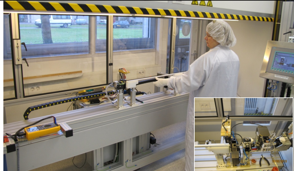
Wire tensioning and crimping + tension measurement
