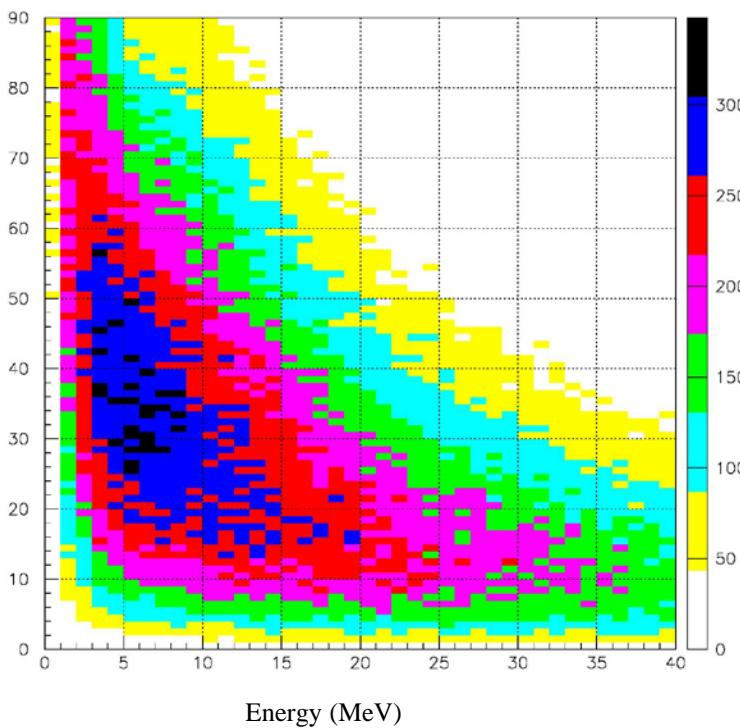
e+ energy [MeV] vs. transverse divergence [deg.] at the production within the e+ capture system acceptance
