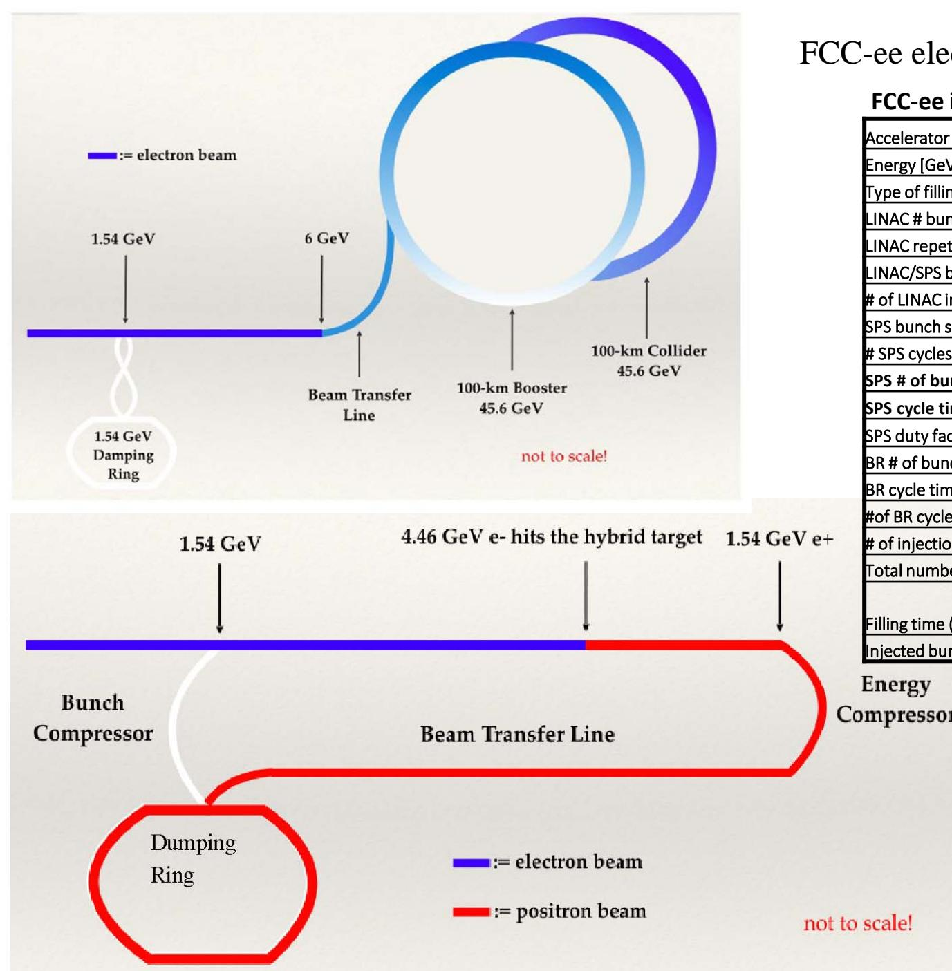
FCC-ee electron flow scheme for Z-pole operation
