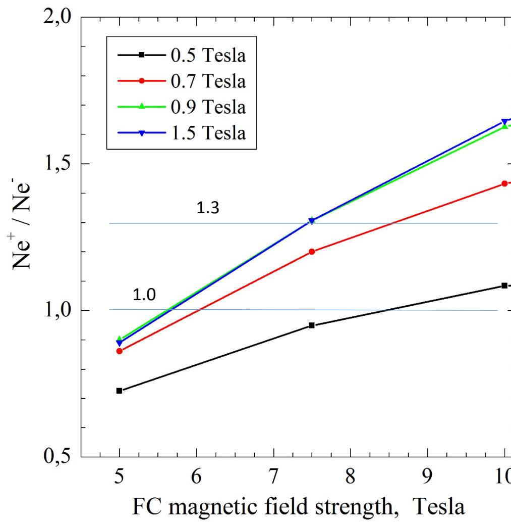
S-band structure linac positron yield after solenoid focusing (250 MeV, with conversion electron bunch energy of 6 GeV)
