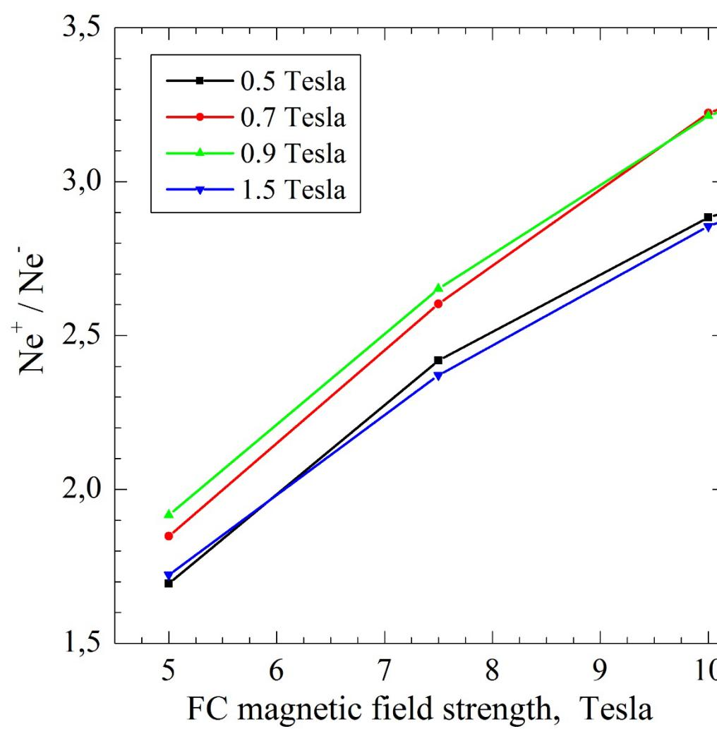
L-band structure linac positron yield after solenoid focusing (250 MeV, with conversion electron bunch energy of 6 GeV)
