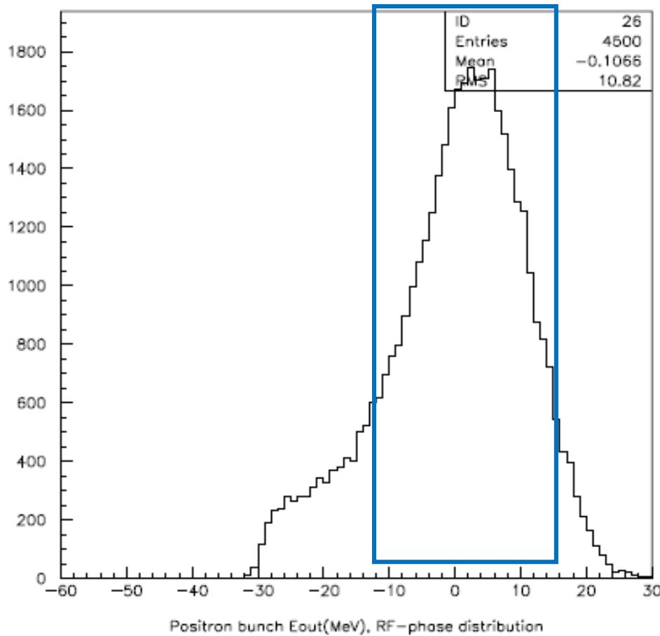
Initial RF phase of accelerating structure is 20 degrees
